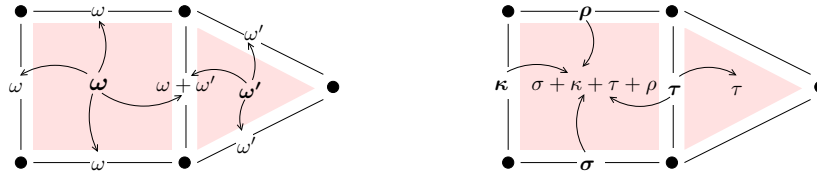
Figure 8: Depiction of the boundary and coboundary operation on chains. We consider the abstract complex already used in figure 7. The effect of taking the boundary operator \partial on \ell_2 = \omega.s + \omega'.s' is pictured by the diagram in the left. The figure in the right gives the effect of taking the coboundary \delta of the 1-chain \ell_1 = \rho.a + \kappa.b + \sigma.c + \tau.d . The coboundary operators \delta^p are the dual homomorphisms of the operators \partial_p (see [17]). In these two figures, the curved arrow indicate values (in bold) being transferred from a p -cell to the preceding (p - 1) -cells (for \partial ) and from a (p - 1) -cell to the succeeding p -cells (for \delta ).
